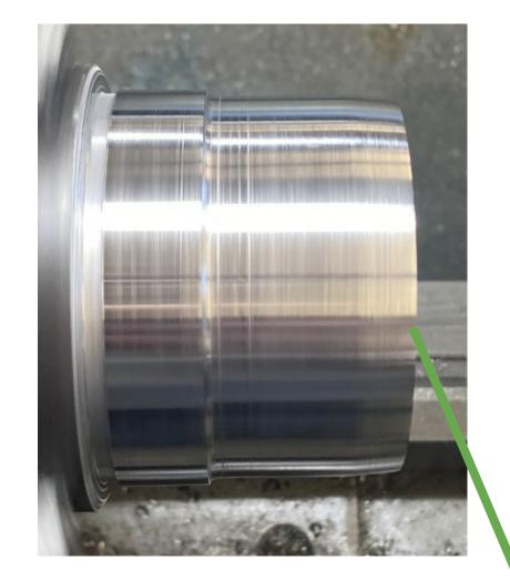
Fabricated custom die to efficiently punch out the correct size of for the thermoformed piece
